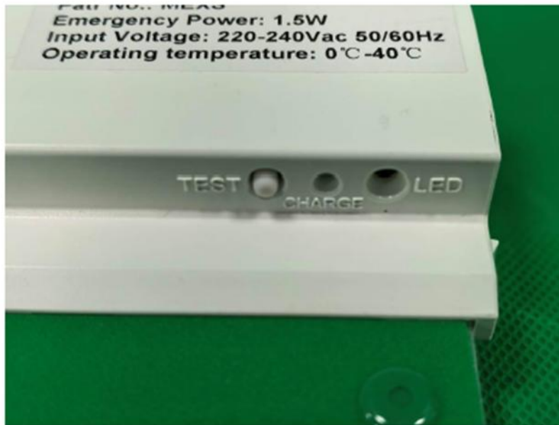
Test switch and indicator for MEXS
