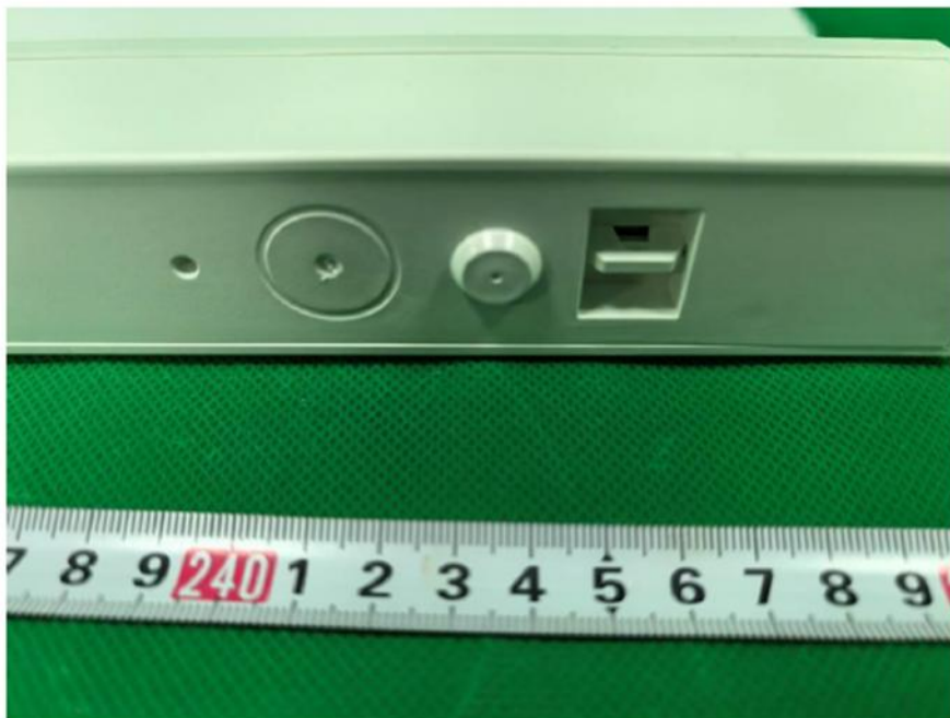
Cable entry and installation hole
